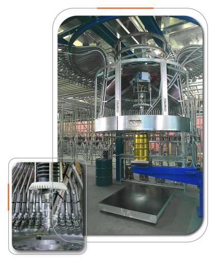
The systems can handle both water based as well as solvent-based products ( ATEX or IEC-EX - version )
